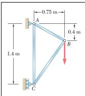
Members AB and BC of the truss shown are made of the same alloy. It is known that a 20-mm-square bar of the same alloy was tested to failure and that an ultimate load of 120 kN was recorded. If a factor of safety of 3.2 is to be achieved for both bars, determine the required cross-sectional area of (a) bar AB, (b) bar AC.
