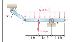
Link AB is to be made of a steel for which the ultimate normal stress is 65 ksi. Determine the cross-sectional area of AB for which the factor of safety will be 3.20. Assume that the link will be adequately reinforced around the pins at A and B.
