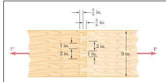
Two wooden planks, each  $\frac{1}{2}$  in. thick and 9 in. wide, are joined by the dry mortise joint shown. Knowing that the wood used shears off along its grain when the average shearing stress reaches 1.20 ksi, determine the magnitude P of the axial load that will cause the joint to fail.
