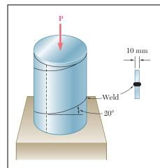
A steel pipe of 400-mm outer diameter is fabricated from 10-mm thick plate by welding along a helix that forms an angle of  $20^{\circ}$  with a plane perpendicular to the axis of the pipe. Knowing that the maximum allowable normal and shearing stresses in the directions respectively normal and tangential to the weld are  $\sigma = 60$  MPa and  $\tau = 36$  MPa, determine the magnitude P of the largest axial force that can be applied to the pipe.
