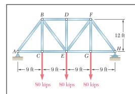
For the Pratt bridge truss and loading shown, determine the average normal stress in member BE, knowing that the cross-sectional area of that member is  $5.87 \text{ in}^2$ .
