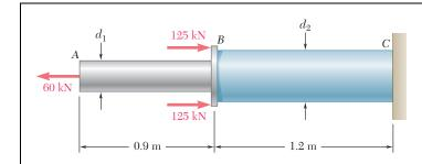
Two solid cylindrical rods AB and BC are welded together at B and loaded as shown. Knowing that  $d_1 = 30$  mm and  $d_2 = 50$  mm, find the average normal stress at the midsection of (a) rod AB, (b) rod BC.
