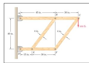
The frame shown consists of *four* wooden members, ABC, *DEF*, *BE*, and *CF*. Knowing that each member has a  $2 \times 4$ -in. rectangular cross section and that each pin has a  $\frac{1}{2}$ -in. diameter, determine the maximum value of the average normal stress (a) in member BE, (b) in member CF.
