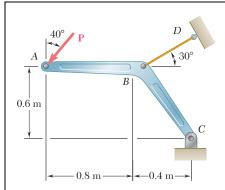
Member ABC, which is supported by a pin and bracket at C and a cable BD, was designed to support the 16-kN load  $\mathbf{P}$  as shown. Knowing that the ultimate load for cable BD is 100 kN, determine the factor of safety with respect to cable failure.
