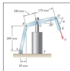
The hydraulic cylinder CF, which partially controls the position of rod DE, has been locked in the position shown. Member BD is 15 mm thick and is connected at C to the vertical rod by a 9-mm-diameter bolt. Knowing that P = 2 kN and  $\theta = 75^{\circ}$ , determine (a) the average shearing stress in the bolt, (b) the bearing stress at C in member BD.
