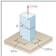
The two portions of member AB are glued together along a plane forming an angle  $\theta$  with the horizontal. Knowing that the ultimate stress for the glued joint is 2.5 ksi in tension and 1.3 ksi in shear, determine (a) the value of  $\theta$  for which the factor of safety of the member is maximum, (b) the corresponding value of the factor of safety. (Hint: Equate the expressions obtained for the factors of safety with respect to the normal and shearing stresses.)
