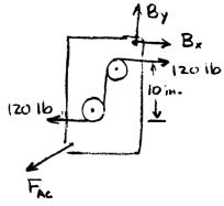
+)\(\Sigma M\_B = 0: -(12 + 4)(F\_{AC}\cos 30^\circ) + (10)(F\_{AC}\sin 30^\circ) - 1200 \text{ lb} = 0\)
