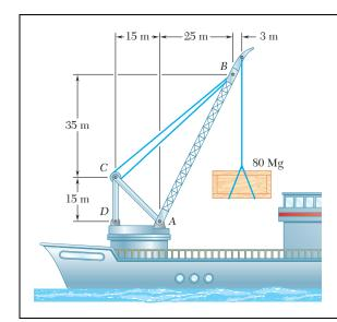
In the marine crane shown, link CD is known to have a uniform cross section of  $50 \times 150$  mm. For the loading shown, determine 'the normal stress in the central portion of that link.
