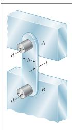
Link AB, of width b = 2 in. and thickness  $t = \frac{1}{4}$  in., is used to support the end of a horizontal beam. Knowing that the average normal stress in the link is -20 ksi and that the average shearing stress in each of the two pins is 12 ksi, determine (a) the diameter d of the pins, (b) the average bearing stress in the link.
