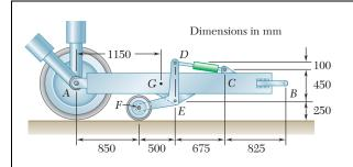
An aircraft tow bar is positioned by means of a single hydraulic cylinder connected by a 25-mm-diameter steel rod to two identical arm-and-wheel units *DEF*. The mass of the entire tow bar is 200 kg, and its center of gravity is located at *G*. For the position shown, determine the normal stress in the rod.
