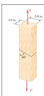
The 1.4-kip load  $\mathbf{P}$  is supported by two wooden members of uniform cross section that are joined by the simple glued scarf splice shown. Determine the normal and shearing stresses in the glued splice.
