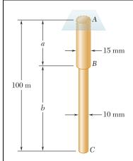
Two brass rods AB and BC, each of uniform diameter, will be brazed together at B to form a nonuniform rod of total length 100 m, which will be suspended from a support at A as shown. Knowing that the density of brass is  $8470 \text{ kg/m}^3$ , determine (a) the length of rod AB for which the maximum normal stress in ABC is minimum, (b) the corresponding value of the maximum normal stress.
