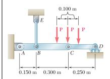
Three forces, each of magnitude P = 4 kN, are applied to the mechanism shown. Determine the cross-sectional area of the uniform portion of rod BE for which the normal stress in that portion is +100 MPa.
