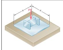
An axial load **P** is supported by a short  $W8 \times 40$  column of cross-sectional area  $A = 11.7 \text{ in}^2$  and is distributed to a concrete foundation by a square plate as shown. Knowing that the average normal stress in the column must not exceed 30 ksi and that the bearing stress on the concrete foundation must not exceed 3.0 ksi, determine the side a of the plate that will provide the most economical and safe design.
