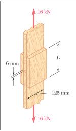
For the joint and loading of Prob. 1.43, determine the factor of safety when L = 180 mm.
