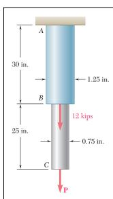
Two solid cylindrical rods AB and BC are welded together at B and loaded as shown. Determine the magnitude of the force  $\mathbf{P}$  for which the tensile stresses in rods AB and BC are equal.
