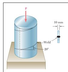
A steel pipe of 400-mm outer diameter is fabricated from 10-mm thick plate by welding along a helix that forms an angle of 20° with a plane perpendicular to the axis of the pipe. Knowing that a 300-kN axial force **P** is applied to the pipe, determine the normal and shearing stresses in directions respectively normal and tangential to the weld.
