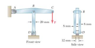
In an alternative design for the structure of Prob. 1.55, a pin of 10-mm-diameter is to be used at A. Assuming that all other specifications remain unchanged, determine the allowable load  $\mathbf{P}$  if an overall factor of safety of 3.0 is desired.
