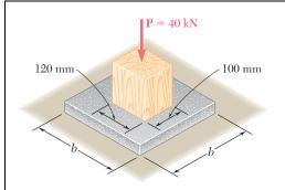
A 40-kN axial load is applied to a short wooden post that is supported by a concrete footing resting on undisturbed soil. Determine (a) the maximum bearing stress on the concrete footing, (b) the size of the footing for which the average bearing stress in the soil is 145 kPa.
