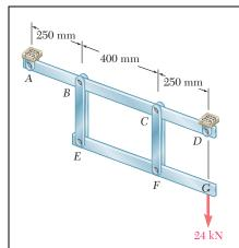
Each of the two vertical links CF connecting the two horizontal members AD and EG has a  $10 \times 40$ -mm uniform rectangular cross section and is made of a steel with an ultimate strength in tension of 400 MPa, while each of the pins at C and F has a 20-mm diameter and are made of a steel with an ultimate strength in shear of 150 MPa. Determine the overall factor of safety for the links CF and the pins connecting them to the horizontal members.
