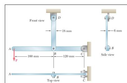
In the steel structure shown, a 6-mm-diameter pin is used at C and 10-mm-diameter pins are used at B and D. The ultimate shearing stress is 150 MPa at all connections, and the ultimate normal stress is 400 MPa in link BD. Knowing that a factor of safety of 3.0 is desired, determine the largest load P that can be applied at A. Note that link BD is not reinforced around the pin holes.
