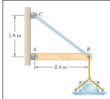
A 40-kg platform is attached to the end B of a 50-kg wooden beam AB, which is supported as shown by a pin at A and by a slender steel rod BC with a 12-kN ultimate load. (a) Using the Load and Resistance Factor Design method with a resistance factor  $\phi = 0.90$  and load factors  $\gamma_D = 1.25$  and  $\gamma_L = 1.6$ , determine the largest load that can be safely placed on the platform. (b) What is the corresponding conventional factor of safety for rod BC?
