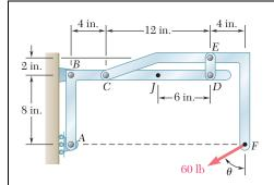
Knowing that the link DE is  $\frac{1}{8}$  in. thick and 1 in. wide, determine the normal stress in the central portion of that link when (a)  $\theta = 0^{\circ}$ , (b)  $\theta = 90^{\circ}$ .
