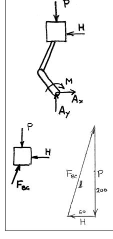
Use piston, rod, and crank together as free body. Add wall reaction H and bearing reactions  $A_x$  and  $A_y$ .
