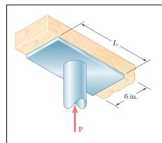
The axial force in the column supporting the timber beam shown is P=20 kips. Determine the smallest allowable length L of the bearing plate if the bearing stress in the timber is not to exceed 400 psi.
