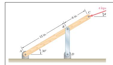
Link BD consists of a single bar 1 in. wide and  $\frac{1}{2}$  in. thick. Knowing that each pin has a  $\frac{3}{8}$ -in. diameter, determine the maximum value of the average normal stress in link BD if (a)  $\theta = 0$ , (b)  $\theta = 90^{\circ}$ .
