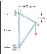
Members AB and BC of the truss shown are made of the same alloy. It is known that a 20-mm-square bar of the same alloy was tested to failure and that an ultimate load of 120 kN was recorded. If bar AB has a cross-sectional area of 225 mm<sup>2</sup>, determine (a) the factor of safety for bar AB and (b) the cross-sectional area of bar AC if it is to have the same factor of safety as bar AB.
