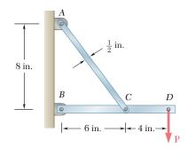
Solve Prob. 1.51, assuming that the structure has been redesigned to use  $\frac{5}{16}$ -in-diameter pins at A and C as well as at B and that no other changes have been made.
