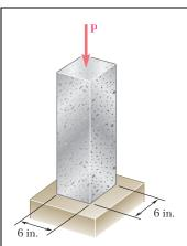
A 240-kip load  $\mathbf{P}$  is applied to the granite block shown. Determine the resulting maximum value of (a) the normal stress, (b) the shearing stress. Specify the orientation of the plane on which each of these maximum values occurs.
