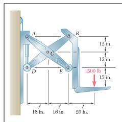
Two identical linkage-and-hydraulic-cylinder systems control the position of the forks of a fork-lift truck. The load supported by the one system shown is 1500 lb. Knowing that the thickness of member BD is  $\frac{5}{8}$  in., determine (a) the average shearing stress in the  $\frac{1}{2}$ -in.-diameter pin at B, (b) the bearing stress at B in member BD.
