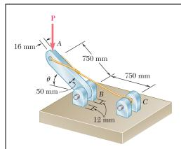
Knowing that  $\theta = 40^{\circ}$  and P = 9 kN, determine (a) the smallest allowable diameter of the pin at B if the average shearing stress in the pin is not to exceed 120 MPa, (b) the corresponding average bearing stress in member AB at B, (c) the corresponding average bearing stress in each of the support brackets at B.
