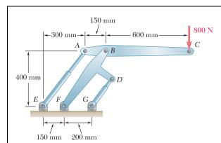
Two hydraulic cylinders are used to control the position of the robotic arm ABC. Knowing that the control rods attached at A and D each have a 20-mm diameter and happen to be parallel in the position shown, determine the average normal stress in (a) member AE, (b) member DG.
