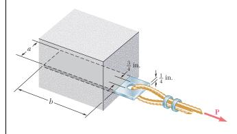
Determine the factor of safety for the cable anchor in Prob. 1.49 when P = 2.5 kips, knowing that a = 2 in. and b = 6 in.
