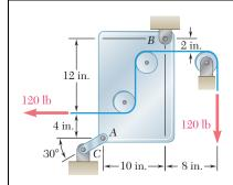
Link AC has a uniform rectangular cross section  $\frac{1}{8}$  in. thick and 1 in. wide. Determine the normal stress in the central portion of the link.
