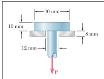
A load P is applied to a steel rod supported as shown by an aluminum plate into which a 12-mm-diameter hole has been drilled. Knowing that the shearing stress must not exceed 180 MPa in the steel rod and 70 MPa in the aluminum plate, determine the largest load P that can be applied to the rod.
