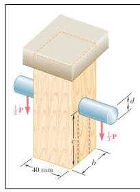
For the support of Prob. 1.47, knowing that the diameter of the pin is d = 16 mm and that the magnitude of the load is P = 20 kN, determine (a) the factor of safety for the pin, (b) the required values of b and c if the factor of safety for the wooden members is the same as that found in part a for the pin.
