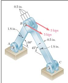
For the assembly and loading of Prob. 1.60, determine (a) the average shearing stress in the pin at C, (b) the average bearing stress at C in member BC, (c) the average bearing stress at B in member BC.
