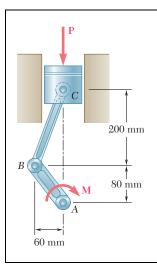
A couple **M** of magnitude 1500 N · m is applied to the crank of an engine. For the position shown, determine (a) the force **P** required to hold the engine system in equilibrium, (b) the average normal stress in the connecting rod BC, which has a 450-mm<sup>2</sup> uniform cross section.
