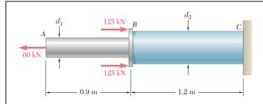
Two solid cylindrical rods AB and BC are welded together at B and loaded as shown. Knowing that the average normal stress must not exceed 150 MPa in either rod, determine the smallest allowable values of the diameters  $d_1$  and  $d_2$ .
