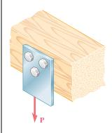
Three steel bolts are to be used to attach the steel plate shown to a wooden beam. Knowing that the plate will support a load P = 28 kips, that the ultimate shearing stress for the steel used is 52 ksi, and that a factor of safety of 3.25 is desired, determine the required diameter of the bolts.
