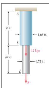
Two solid cylindrical rods AB and BC are welded together at B and loaded as shown. Knowing that P = 10 kips, find the average normal stress at the midsection of (a) rod AB, (b) rod BC.
