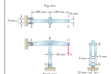
In the structure shown, an 8-mm-diameter pin is used at A, and 12-mm-diameter pins are used at B and D. Knowing that the ultimate shearing stress is 100 MPa at all connections and that the ultimate normal stress is 250 MPa in each of the two links joining B and D, determine the allowable load P if an overall factor of safety of 3.0 is desired.
