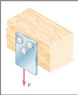
Three  $\frac{3}{4}$ -in.-diameter steel bolts are to be used to attach the steel plate shown to a wooden beam. Knowing that the plate will support a load P = 24 kips and that the ultimate shearing stress for the steel used is 52 ksi, determine the factor of safety for this design.
